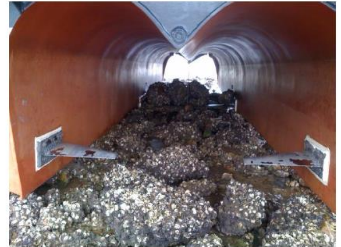
11m HYSUCAT hit rocks at 30 knots. No damage to foils!! Vessel went back into service the next day.
